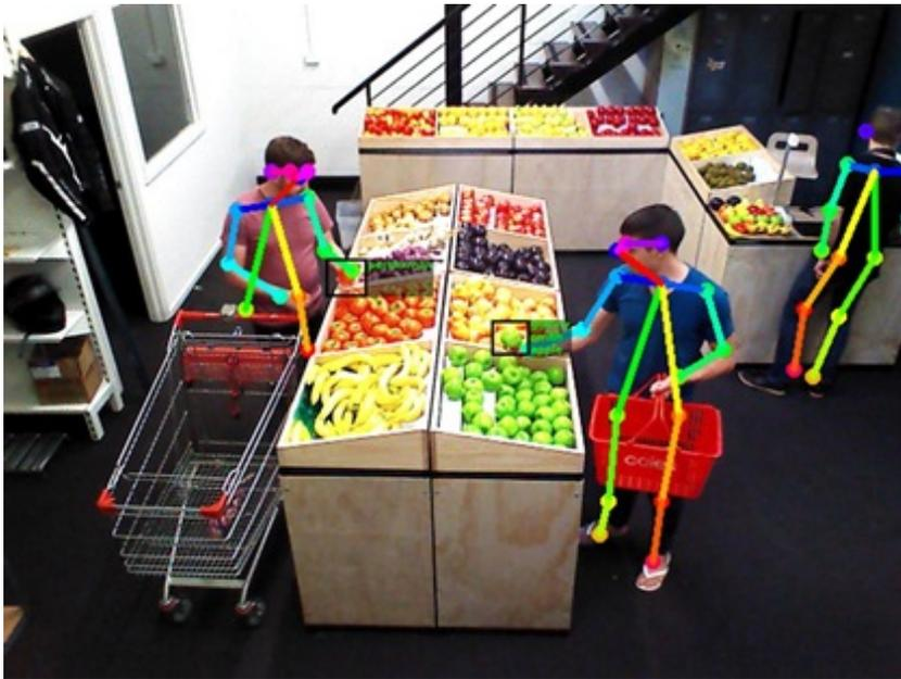
Taking loss prevention technology one step further, Australian startup black.ai has developed a platform which uses 3D sensors to maintain a 'virtual cart' of items for each customer. The artificial intelligence platform detects the products a customer has picked up and put back, including fresh produce. It can even determine whether a shopper has placed a Granny Smith or a Pink Lady in their basket, and can figure out whether a customer is attempting to trick a self-scan checkout.
